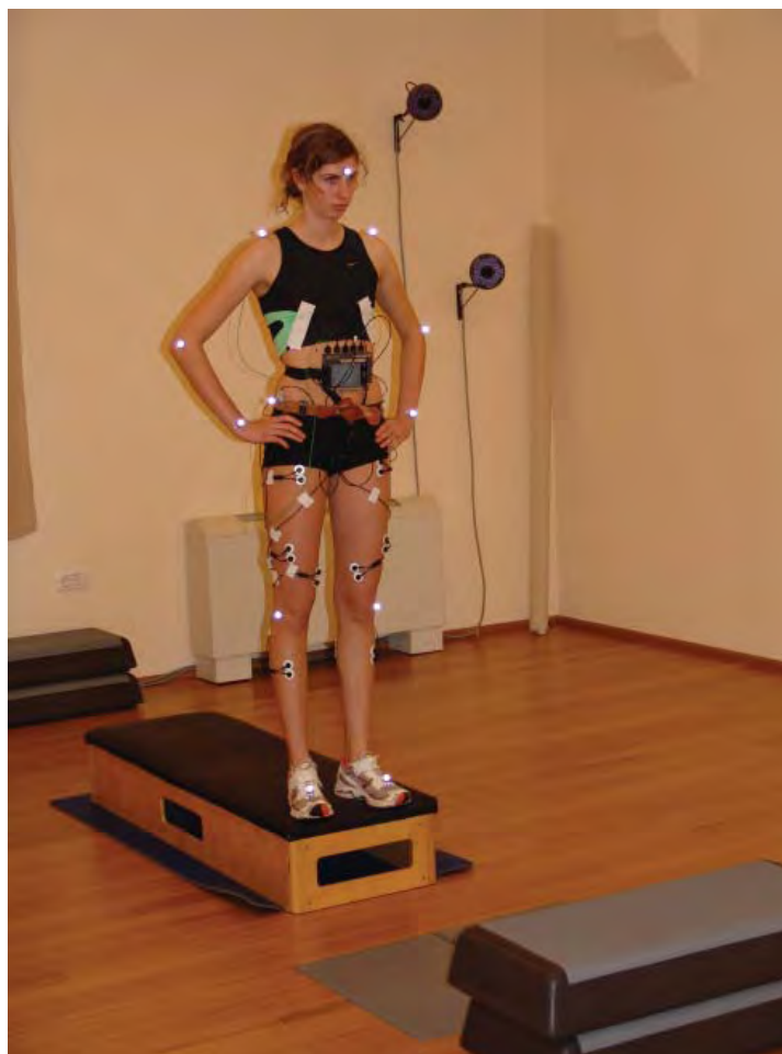
Figure 1. Measurement protocol for kinematic, dynamic and EMG parameters (drop jump)
